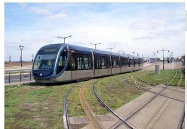
**Light Rail/Diesel Multiple Unit** – A rail transit line that can operate in a variety of settings including dedicated ROW, subway, or mixed on-street traffic. Light rail transit (LRT) usually relies on overhead wires for power and is designed for heavily traveled corridors where the stop needs do not support heavy rail transit, and are typically not compatible with freight rail.
