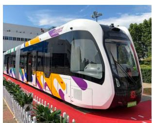
**Autonomous Road Train** – An emerging vehicle technology that combines the capacity and form-factor of a traditional streetcar with rubber-tire operation. Manufacturers are planning for the incorporation of advanced autonomous and connected technology, essentially providing a rail-type service, without the cost associated with rail infrastructure.
