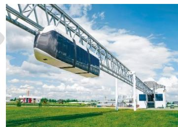
**String Rail** - A future concept using rigid overhead rails to transport passenger pods of various sizes. Unlike PRT, these systems would operate similar to traditional transit, and board at every stop. No functioning system has yet to be fully deployed for commercial or public use at this time.
