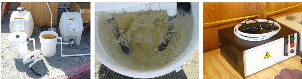
Figure 9. Passive ozonation tank and the aeration tubes (left and center), and the ozone generator located within the field laboratory (right).
