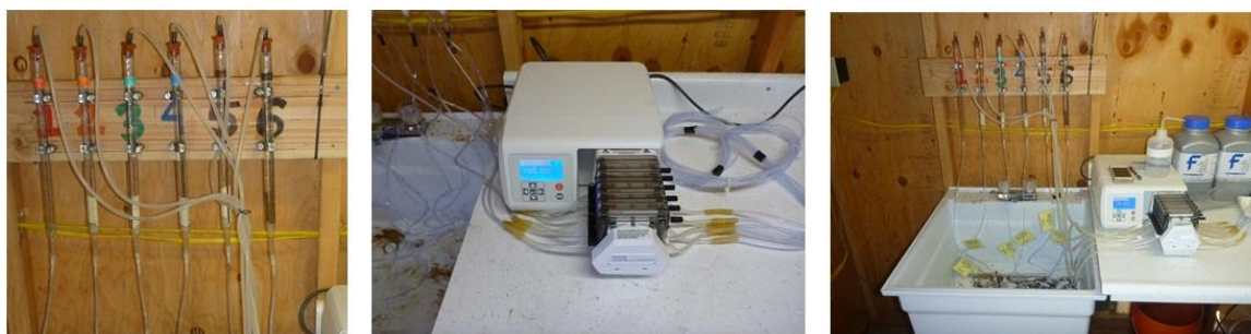
Figure 10. Polymorphic bead filtration manifold with five bead types (2-6) and a single control tube (1), and programable six channel peristaltic metering pump.
