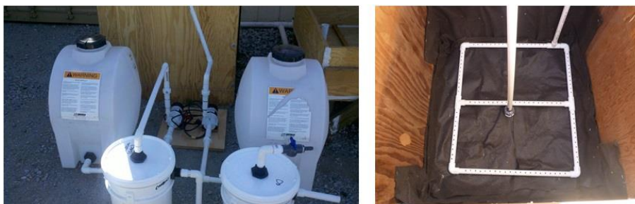
Figure 7. Intermediate storage tanks used for lake water collection (left) and the back-flushing manifold used to clean the filtering sand using fresh water (right). The back-flushing manifold was placed on permeable cloth above the layer of gravel (Figure 5).
