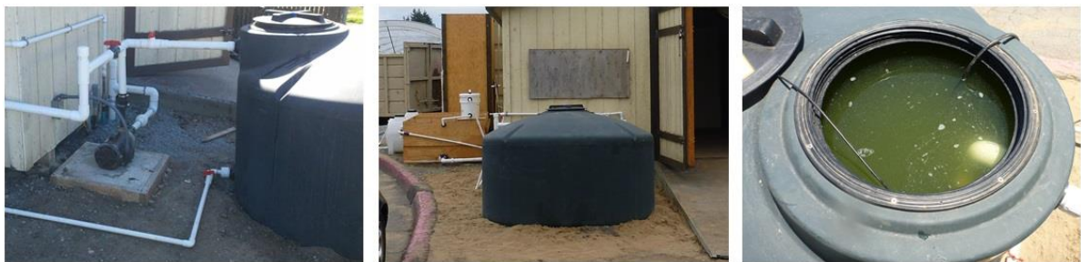
Figure 3. Water was pumped from the lake to a storage tank located outside the field laboratory for each experimental run. Water within the tank was circulated with a submersible pump during each experimental run to ensure uniform bacterial distribution throughout the run.
