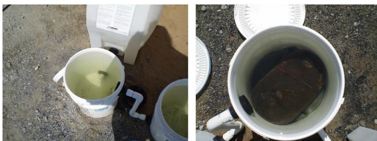
Figure 8. Passive Granular Activated Carbon (GAC) filtration tank (left) and GAC contained within a fine mesh bag.
