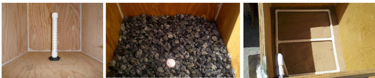
Figure 6. Interior of the slow sand filter, showing the outflow manifold (left), the bed of gravel (center), the inflow manifold and the bed of sand used to filter the lake water (right).
