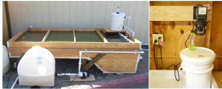
Figure 4. The settling tank, showing the inlet manifold, the settling trough, the laminar baffle, the two surface skimmers, and the standpipe drain (left). Lake water from the storage tank was pumped into the alum mixing tank where a predetermined concentration of alum was added using a paristaltic metering pump (right).
