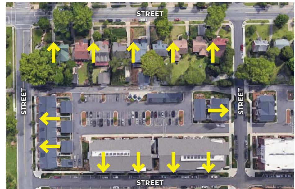
**BUILDING PLACEMENT**—This example block shows buildings sited and oriented (with yellow arrows representing building orientation) to define and engage streets, with parking to the rear of buildings.
